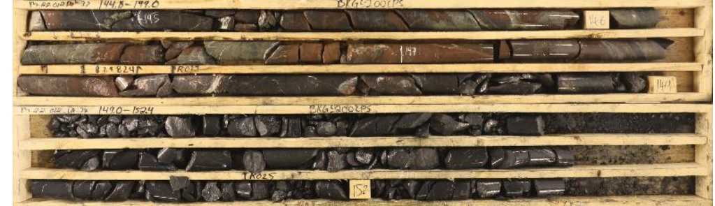
M22-012 (target H11): Hydrothermal hematite (oxidation front) at 147 m in contact with strongly graphitic pelite with significant faulting.
