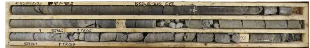
M22-014 (target P1): Strong hydrothermal clay development within fault zone from 93 to 96 m including core loss.
