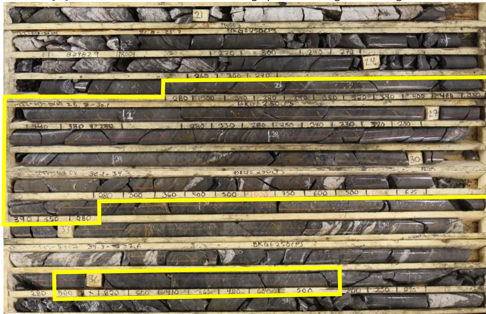
M22-013 (target P1): Graphitic pelite with patchy hematization, including 653 ppm U from 30.8 to 30.9 m associated with fractures, shearing, localized quartz flooding and elevated pyrite content.
