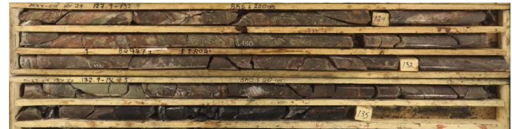
M22-015 (target A10): Structurally-controlled hydrothermal hematite and strong alteration from 127.9 m above faulted graphitic pelite at 134.3 m.
