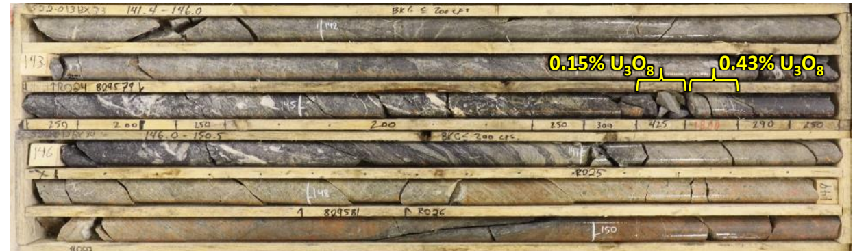
Drill hole S22-013: Uranium mineralization in favorable graphitic fault with alteration
