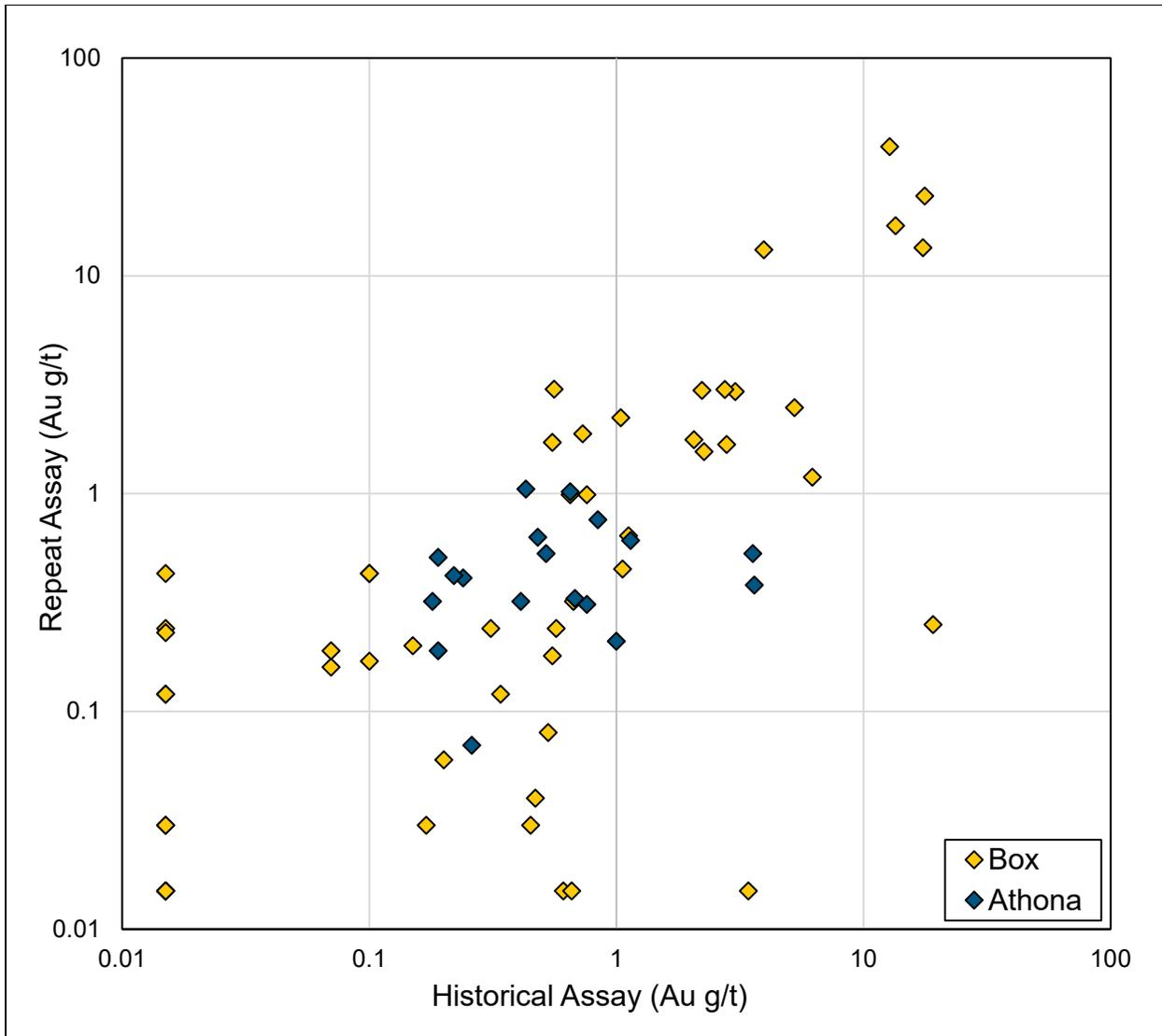
**Figure 1: Plot showing gold assay results from 70 historical drill core samples (half NQ core predominantly over 1 m increments) in comparison with repeat assay results for the remaining half core over the same sample intervals.**
