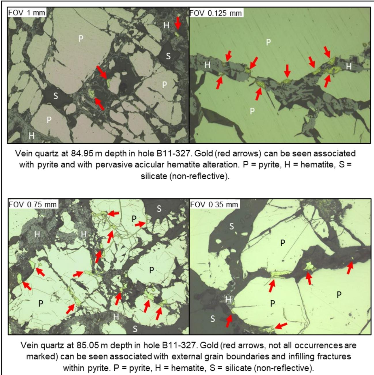
**Figure 2: Photomicrographs (reflected PPL) of polished thin sections from historical drill core prepared from the Box Deposit high grade core.**
